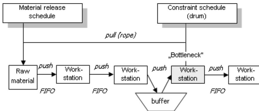
**Fig. 1** The idea of Drum-Buffer-Rope methods (Hadaś & Cyplik, 2010)
