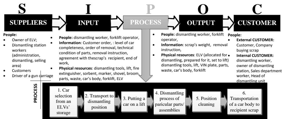
Fig. 3 SIPOC diagram for dismantling an ELV process
