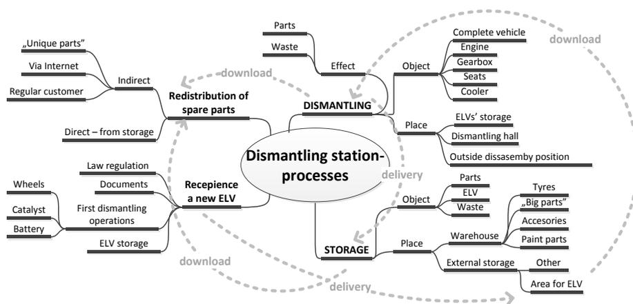
Fig. 2 Process in dismantling station
