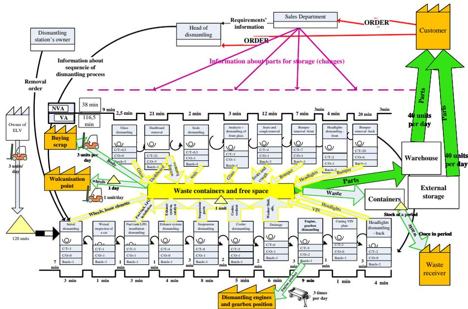
Fig. 5 Value Stream Map for dismantling ELV – at present
