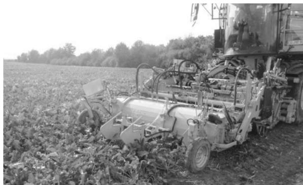
**Fig. 2** Beet harvester – method defoliating (Source: RoPa, 2012)
