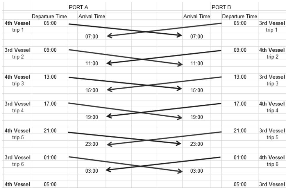
Fig. 3 Time schedule and Operation Time Table for 3rd & 4th RoRo vessel
