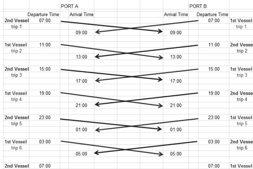
Fig. 2 Time schedule and Operation Time Table for RoRo vessel
