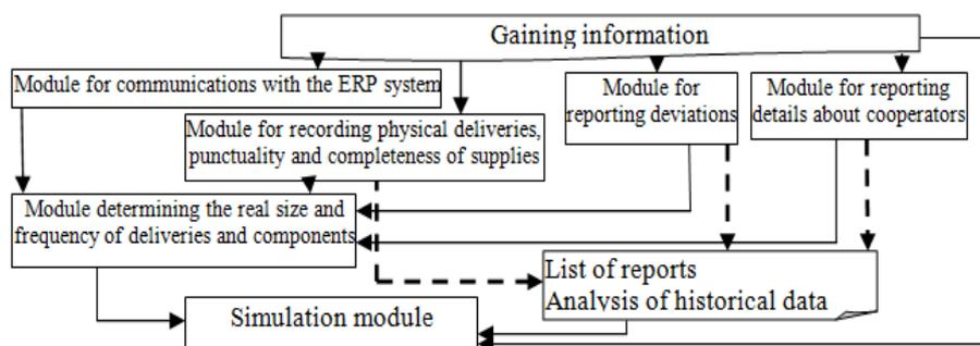
**Fig. 2** Modules of the tool Planning supplies of components and controlling the level of material supplies. Source: The authors' study
