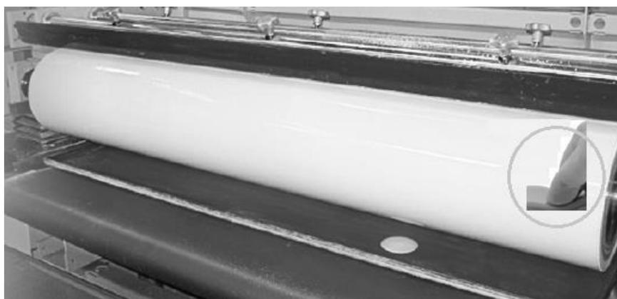
**Fig. 6** Roller coater armed with polyurethane shaft (Szwedzka, 2014)
