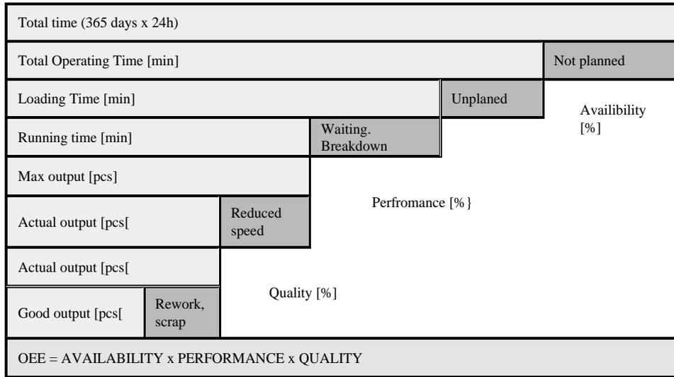
**Fig. 2** The OEE elements connected with the losses
