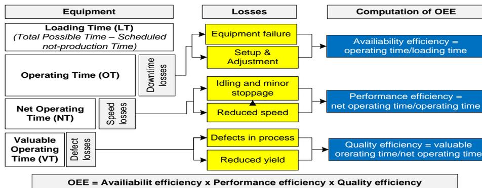
**Fig. 1** Computation of OEE (for individual equipment) (Nakajima, 1988)
