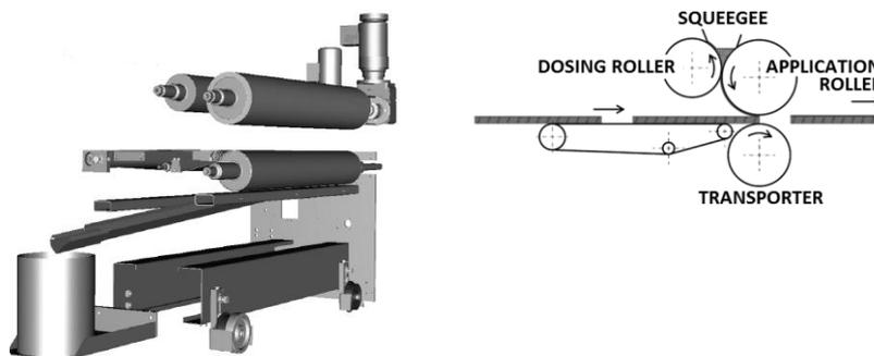
**Fig. 5** Roller applicators scheme and way of the lacquer application process
