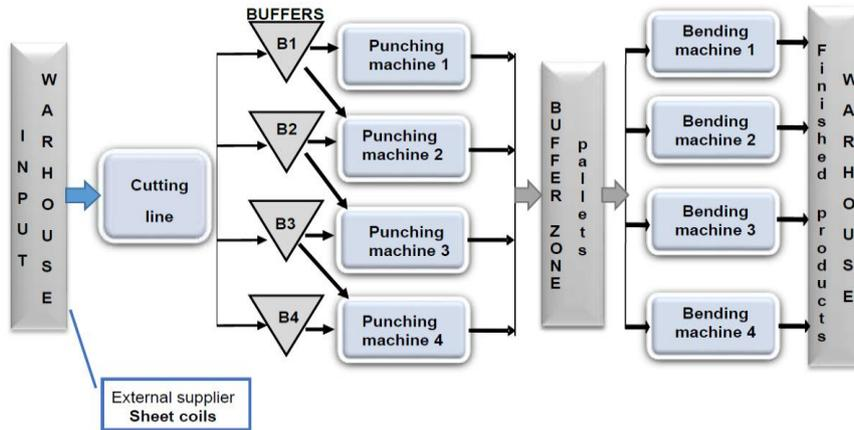
Fig. 4. The structure of the technological process
