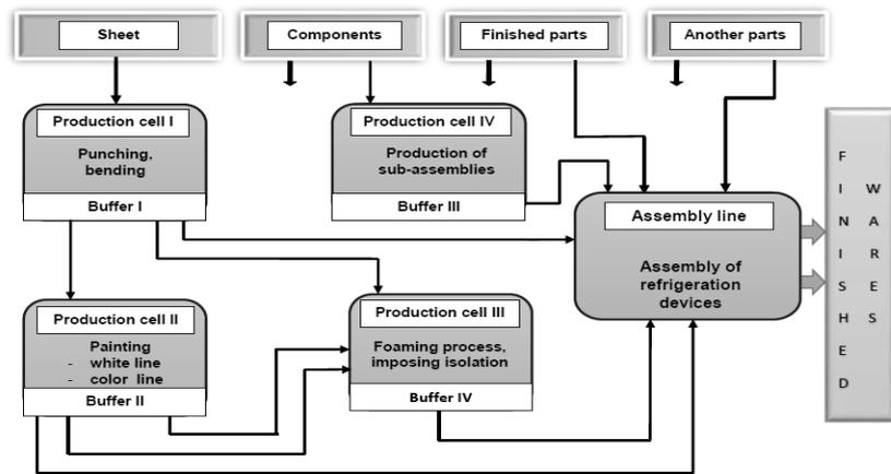
Fig. 1. Scheme of production system
