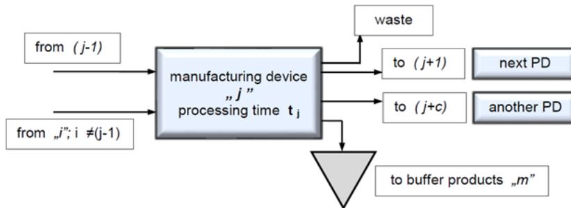
Fig. 2. Scheme of material flow through the manufacturing device PD
