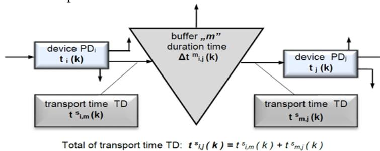
Fig. 3. Diagram of material flow through the buffer
