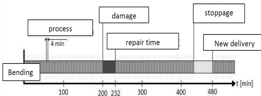
Fig. 8. The schedule of working time, damages and stoppages of workstation
