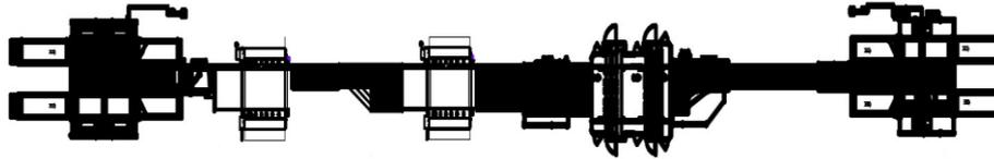
**Fig. 2.** Double-end tenoner line (forming line) for panels processing (in order: feeder, double-end tenoner, turning unit, double-end tenoner, conveyor, drilling machines, conveyor, stacker)
