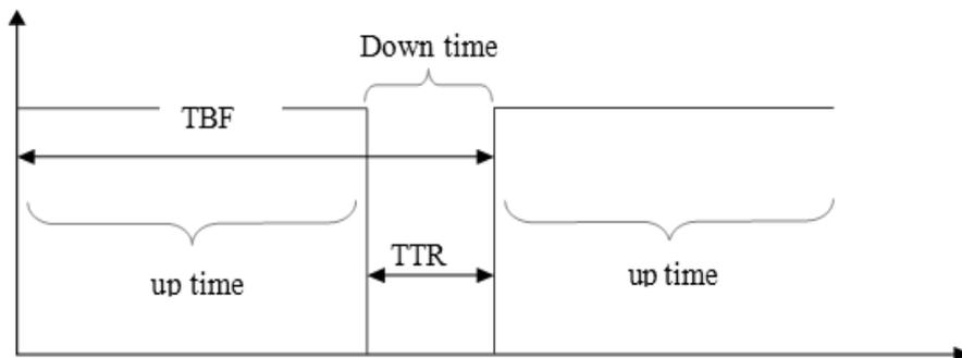
Fig. 1. Calculation of MTBF (TBF – Time Between Failures, TTR – Time To Repair)
