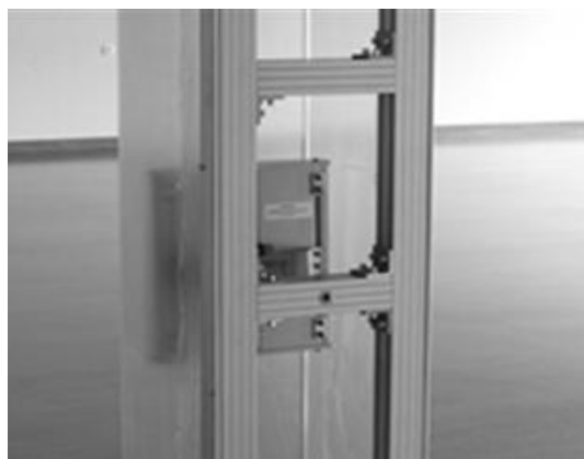
Fig. 1. Element of a gate with an RFID antenna
